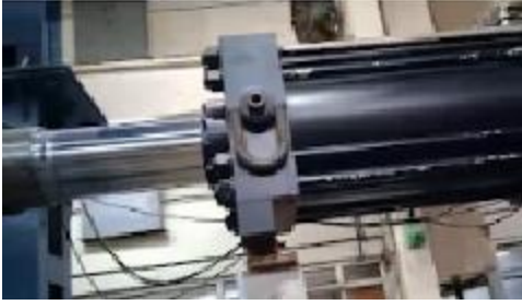
Actuator: Servo Controlled. Make MTS
